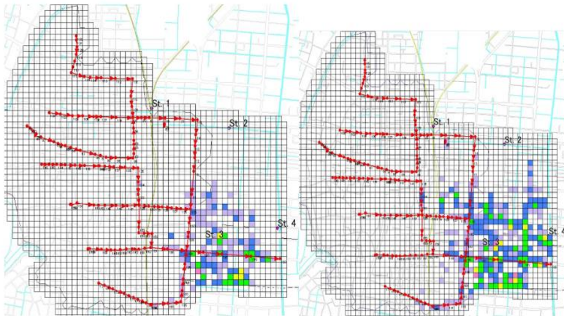
Figure 4.7 Computed inundation depth distributions with (left) and without (right) drainage channel network on the map with sewer system network (red arrows and plots), at 3am October23,2017 in the severest situation
