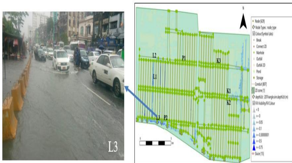
Figure 2.12 Flood condition near Logger ID-L3: A comparison between the inundation map provided by ICM software and an image taken during the event on 2 August 2019
