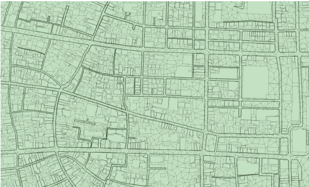
Figure 5.4 Flexible unstructured mesh with triangular cells representing the streets and pervious areas (shown with shadows) of the city. Building areas are excluded by 2D domain
